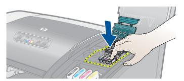
7 Close the printhead access latch firmly, ensuring the hook catches the carriage lock, and then close the printing supplies cover. You will need to use some force to close the printhead access latch.
